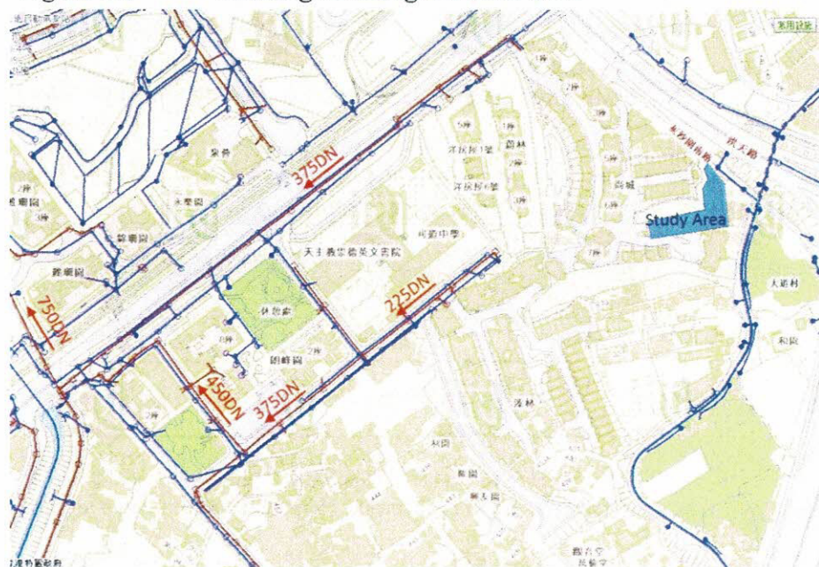
Figure 2.1 Existing Sewerage Record Plan
